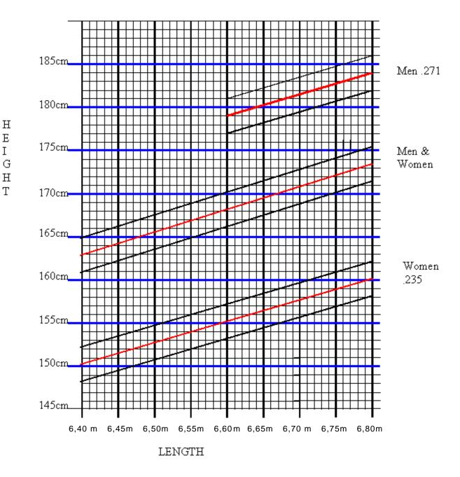
Instructions: For any particular ramp setting, a combination of HEIGHT at the top edge and LENGTH out of the water enclosed within the solid line is allowable. A combination that lies on the dotted (middle) line is the most desirable.
